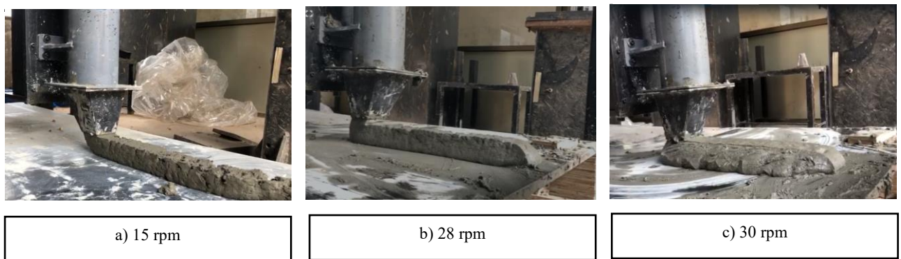
Figure 4.3: Printed mix at different extrusion speeds as follows: a) 15 rpm, b) 28rpm, c) 30 rpm
