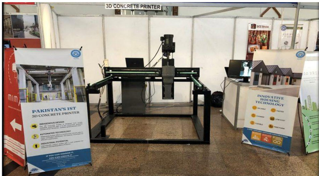
Figure 2-16: 3D Concrete Printer Prototype (mmnews, 2023)
