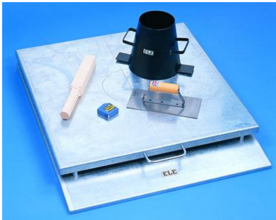
Figure 2-11: Flow table apparatus (ELE International, 2024)
