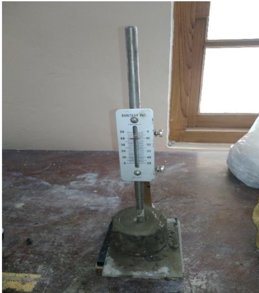
Figure 3-2 Consistency Test with Vicat Apparatus
