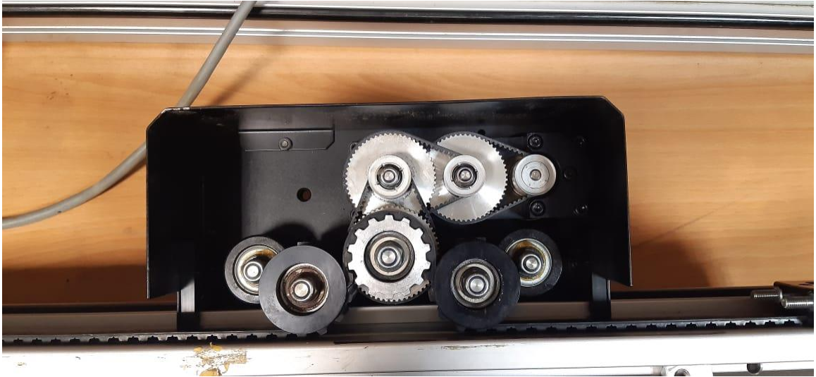
Figure 9: Gearbox of the Linear Actuators
