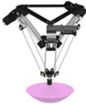
Figure 6: Delta Robot with 3 Linear Actuator at an angle
