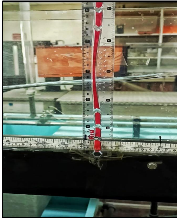
Figure 3.15: Horizontal as well as vertical scale with the help of which difference in wave parameters are quantified.
