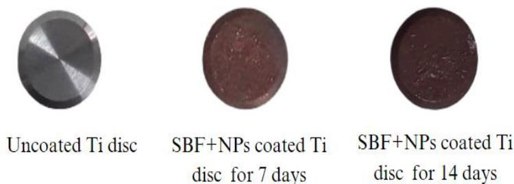
**Figure 4. 11:** Images of uncoated titanium disc, disc coated for 7 and 14 days
