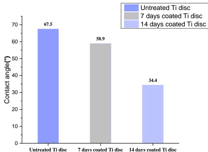
**Figure 4. 18:** Graphical representation of comparison of contact angle for untreated Ti disc, 7 days and 14 days coated Ti discs
