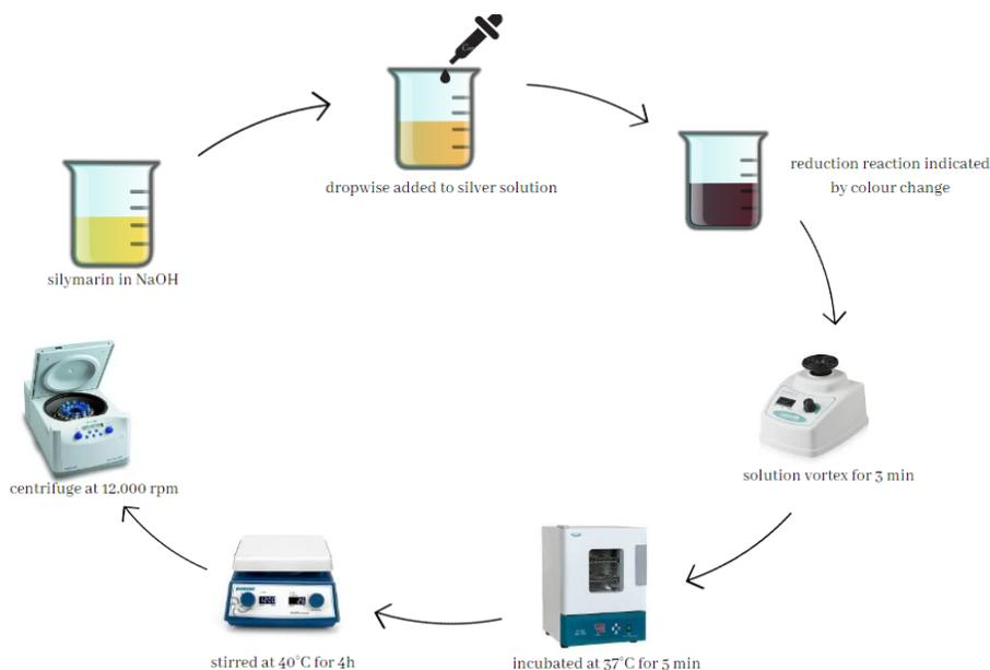
**Figure 3. 1:** Flow diagram showing the stepwise protocol for silver nanoparticles synthesis
