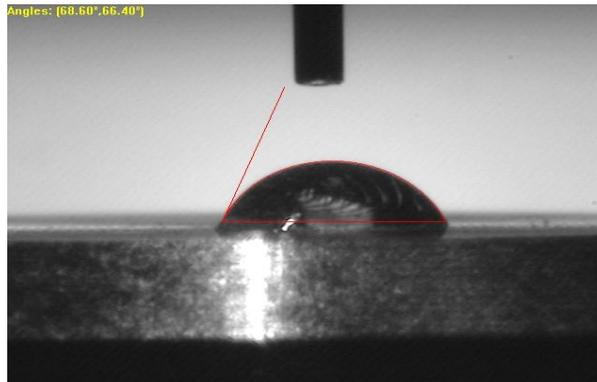
**Figure 4. 15:** left and right contact angle for untreated Ti disc
