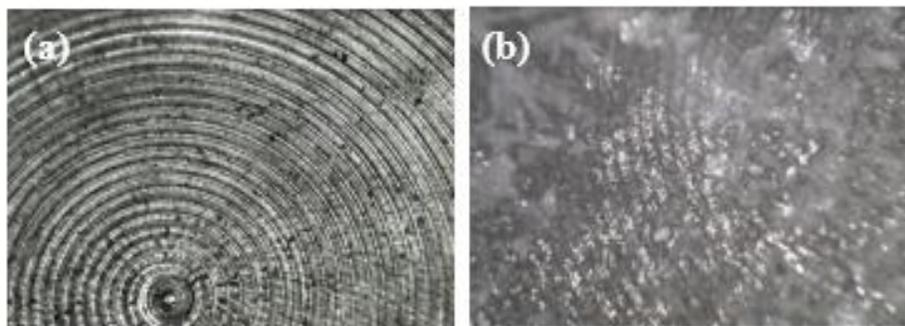
**Figure 4. 12:** Images of untreated Ti disc under optical microscope at 5x magnification. Image of uncoated titanium disc (a), image of titanium disc after alkaline treatment (b)
