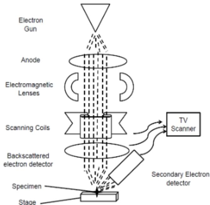
**Figure 3. 4:** Working principle of scanning electron microscope
