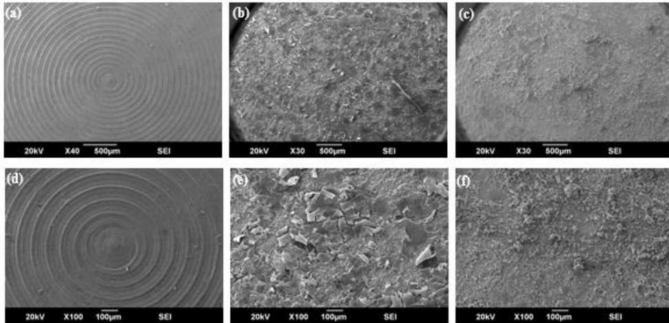
**Figure 4. 14:** SEM Images of uncoated Ti disc, Ti disc coated for 7 days and Ti disc coated for 14 days at scale bar 500 and 100 μm. Uncoated disc at scale bar 500 μm (a), 7 days coated disc at scale bar 500 μm (b), 14 days coated disc at scale bar 500 μm (c), uncoated disc at scale bar 100 μm (d), 7 days coated disc at scale bar 100 μm (e), 14 days coated disc at scale bar 100 μm (f)
