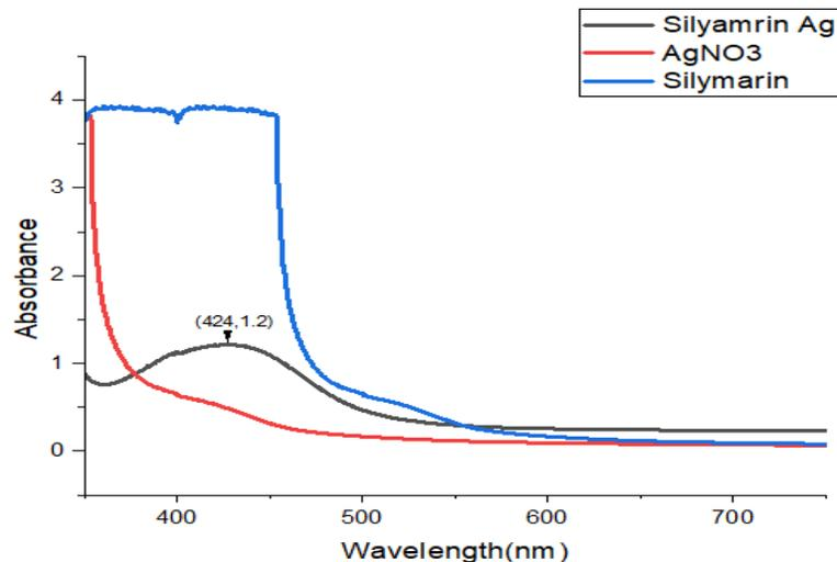
**Figure 4. 1:** UV Spectrum of Silymarin Silver Nanoparticles
