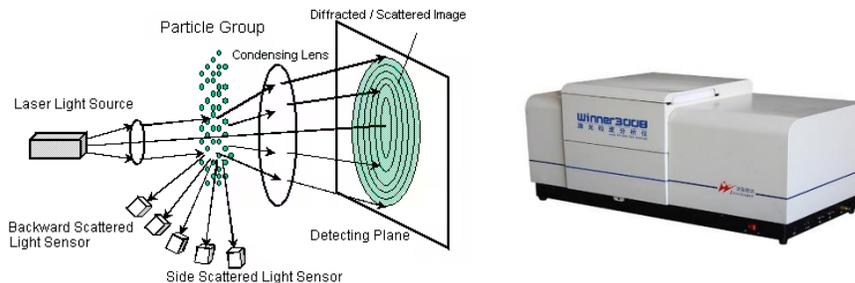
**Figure 3. 7:** Laser diffraction particle size distribution analyzer
