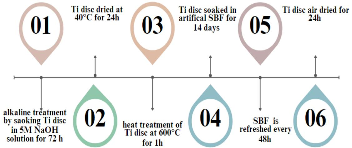
**Figure 3. 2:** Flow diagram showing the process of Ti disc coating with SBF and nanoparticles
