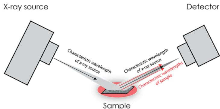
**Figure 3. 6:** Representation of XRD working principle
