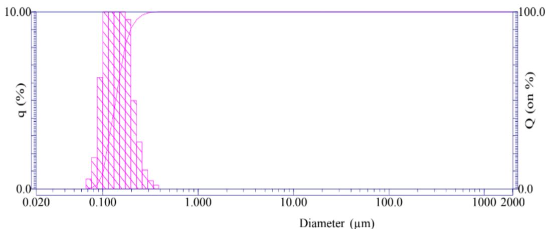
**Figure 4. 10:** Particle size distribution of Silymarin Silver Nanoparticles
