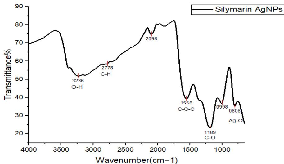
**Figure 4. 3:** FTIR Analysis of Silymarin Silver Nanoparticles
