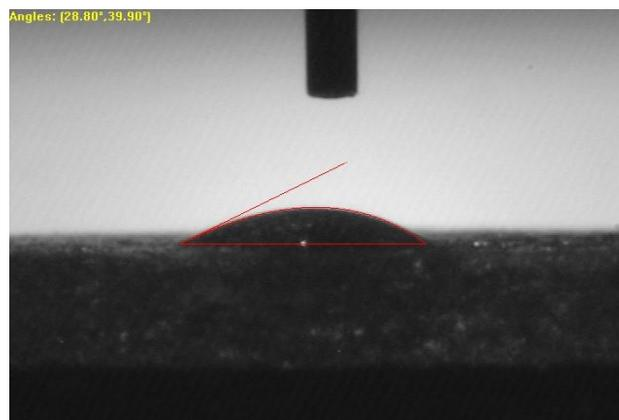
**Figure 4. 17:** Left and right contact angle for Ti disc coated for 14 days
