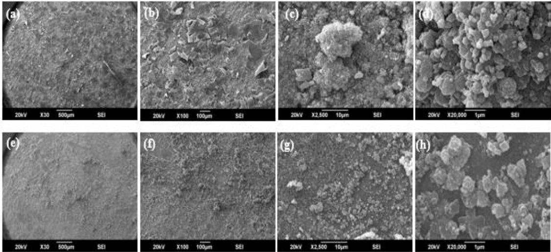
**Figure 4. 13:** SEM Images of 7 and 14 days coated Ti disc at scale bar 500, 100, 10 & 1 μm. 7 days coated disc at scale bar 500 μm (a), at scale bar 100 μm (b), at scale bar 10 μm (c), at scale bar 1 μm (d), 14 days coated disc at scale bar 500 μm (e), at scale bar 100 μm (f), at scale bar 10 μm (g), at scale bar 1 μm (h)
