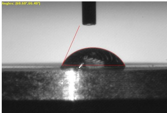
**Figure 4. 16:** Left and right contact angle for Ti disc treated for 7 days
