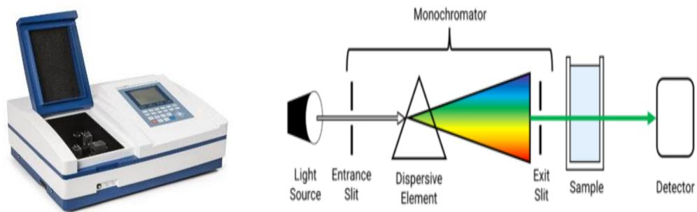
**Figure 3. 3:** UV spectrophotometer and its working principle
