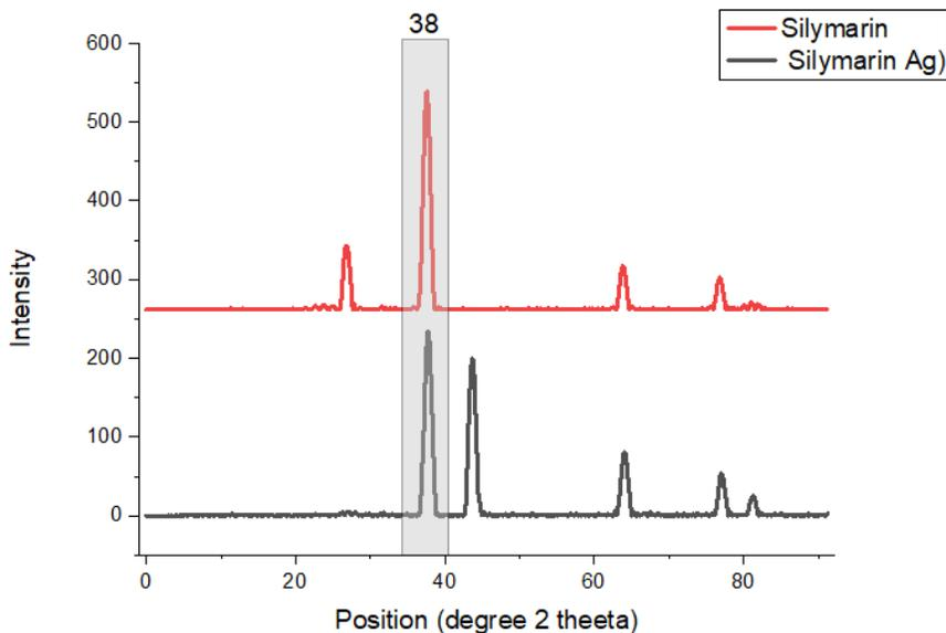
**Figure 4. 8:** Comparison of XRD spectra for Silymarin & Silymarin Silver Nanoparticles
