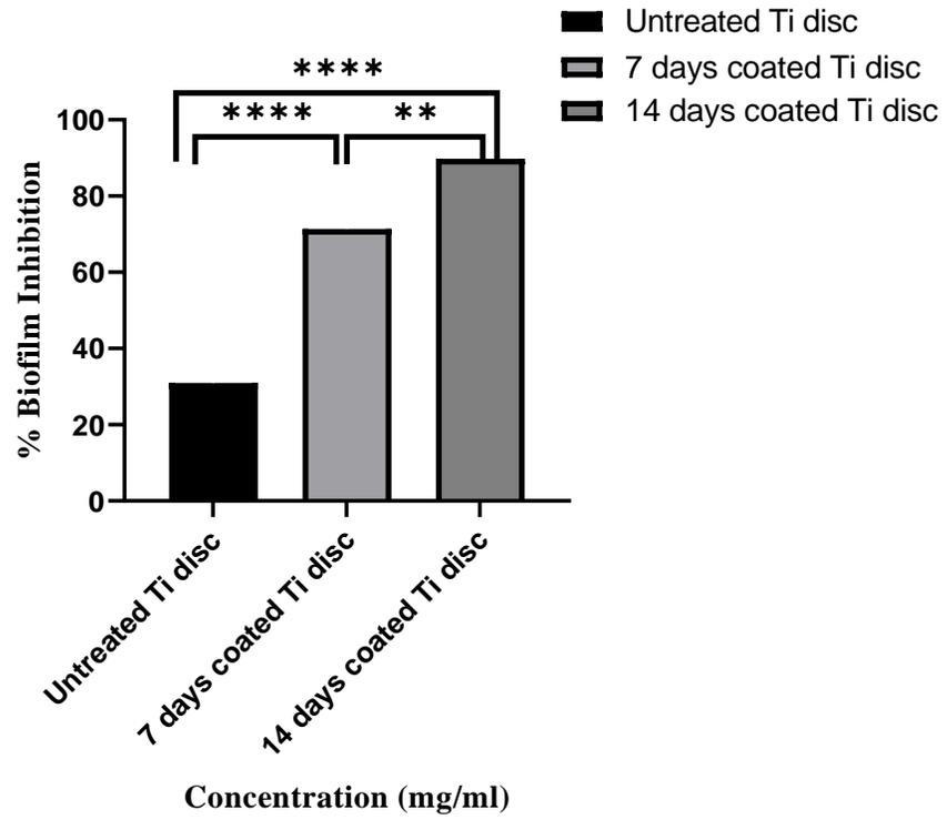
**Figure 4. 19:** Comparison for anti-biofilm activity of untreated Ti disc, disc coated for 7 days and disc coated for 14 days at p value<0.0001
