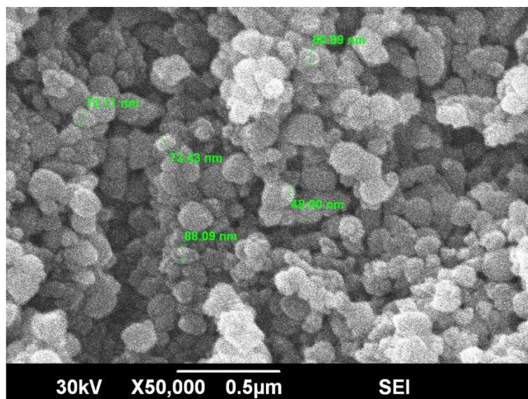
**Figure 4. 2:** SEM Analysis of Silymarin Silver Nanoparticles at scale bar of 0.5μm
