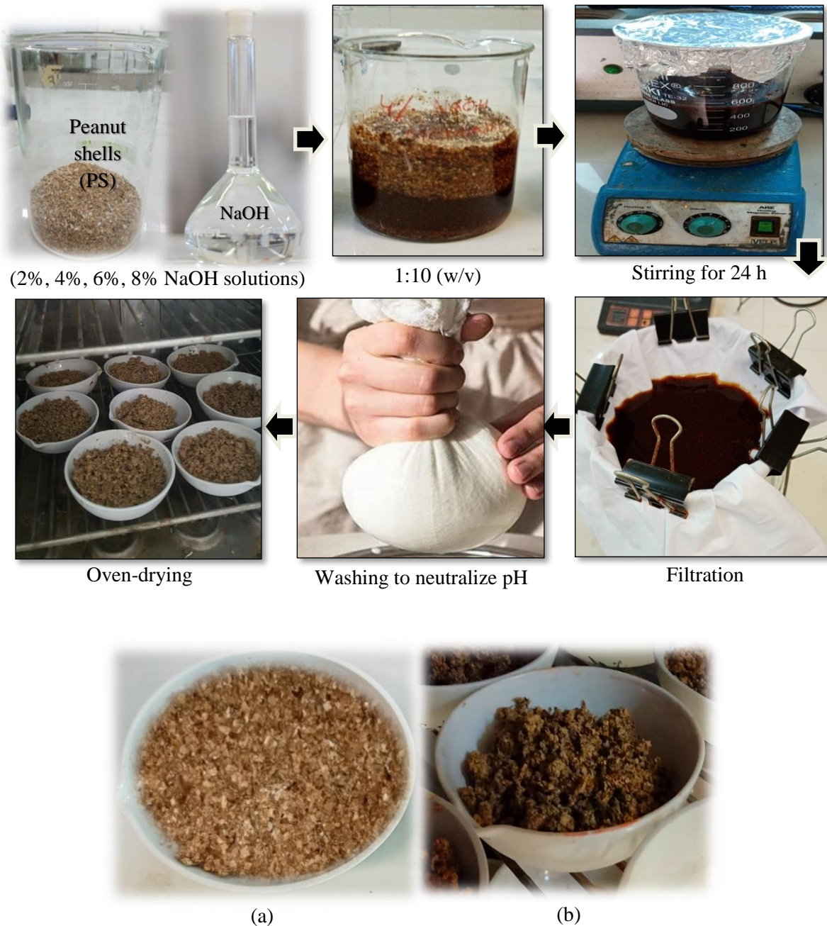
Figure 3.6 Alkaline pretreatment of peanut shells: (a) Untreated PS (b) Pretreated PS
