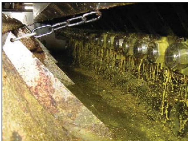
Figure 3.8 Oil flowing between cage bars. Courtesy of Desmet Rosedowns. The full colour version can be found on the plates.
