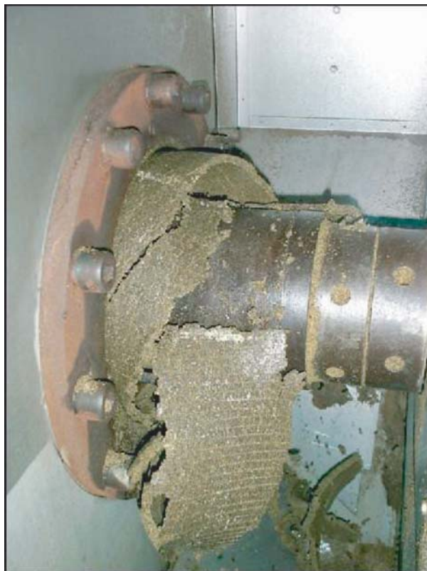
Figure 3.9 Pressed cake at outlet. Courtesy of Desmet Rosedowns. The full colour version can be found on the plates.
