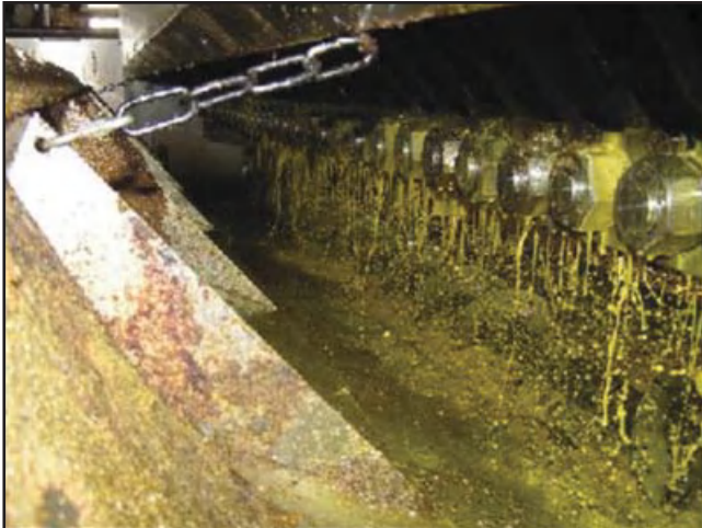
Plate 3.8 Oil flowing between cage bars. Courtesy of Desmet Rosedowns.
