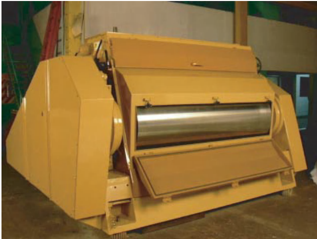
Plate 3.2 Industrial flaking mill. Courtesy of Allocco.
