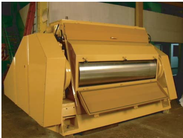
Figure 3.2 Industrial flaking mill. Courtesy of Allocco. The full colour version can be found on the plates.
