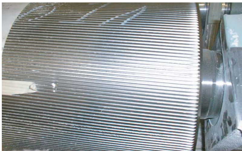
Figure 3.1 Detail of a corrugated roll in a cracking mill. Courtesy of Allocco. The full colour version can be found on the plates.
