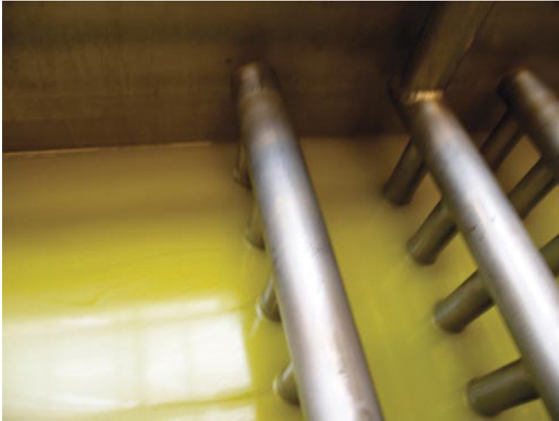
Plate 6.10 Detail of MoBulizer™ cooling tubes in vegetable oil.
