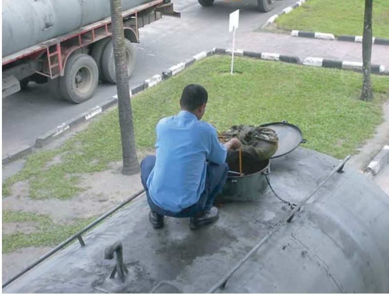
Figure 10.15 Unsafe top access to a road tanker.
