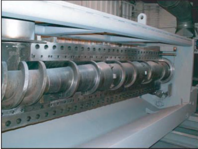
Plate 3.7 Typical worm assembly, showing worms, distance pieces, knife bars and a mixing device. Courtesy of Desmet Rosedowns.
