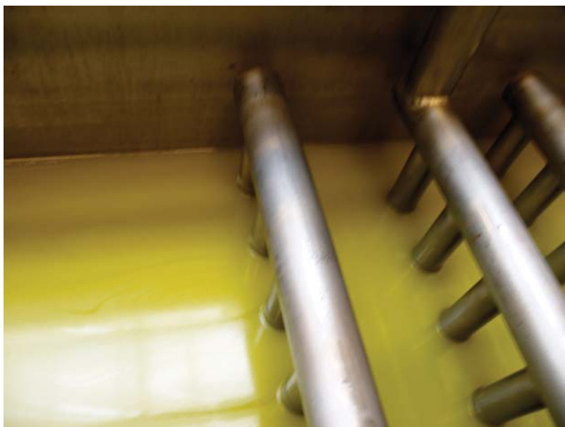
Figure 6.10 Detail of MoBulizer™ cooling tubes in vegetable oil. The full colour version can be found on the plates.
