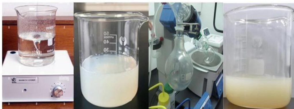
Figure 12: the mixing of lipid solution and thymol(A) thick suspension after mixing (B) rotary evaporation(C) liposomes after filtration (D)
