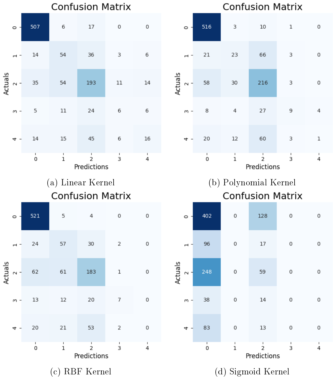
Figure 4.5: Confusion matrix shows correct and incorrect classifications made by the classifier, where diagonal elements represents right predictions and non-diagonal elements denotes misclassifications.
