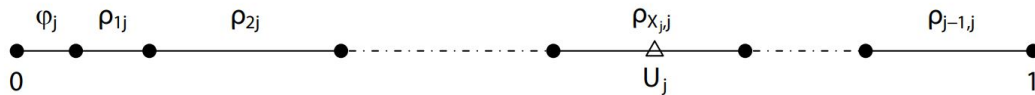
Figure 1.1: Algorithmic representation of stochastic declustering depicts the random classification of earthquake clusters, showing the computation of \phi_j and \rho_{ij} for every event j , creating a random variable U_j , and deciding the classification of event j depending on the total impact of previous events. This procedure determines if an event is part of the background or a child event in the cluster.
