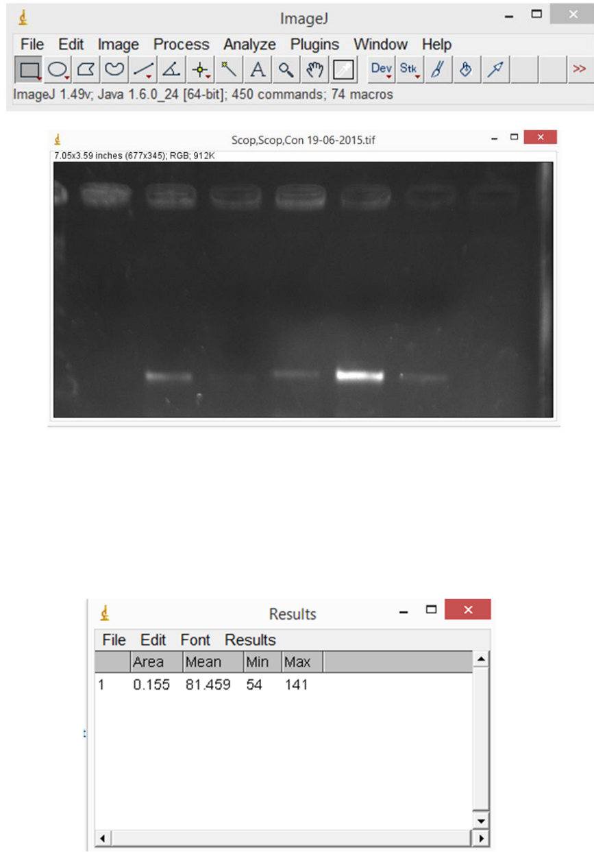
Figure 5: User interface of NIH software ImageJ used for quantification of band intensities. Gel image with a selected band and subsequent value of band intensity is shown in the results window.
