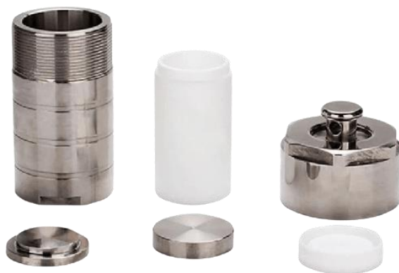
Figure 9: Stainless steel autoclave with Teflon beaker generally used for solvothermal or hydrothermal synthesis
