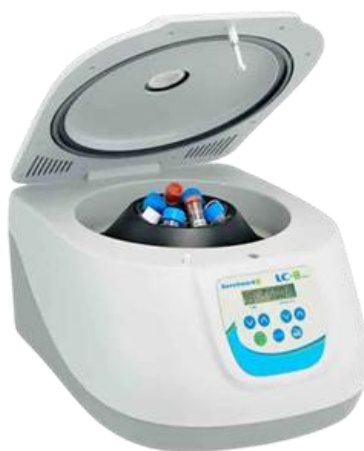
Figure 11: Centrifuge machine used for washing process after hydrothermal synthesis.
