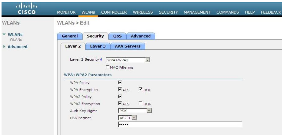
Figure 5.3.2(3-b): WLC Configuration for WLAN Communication Security
