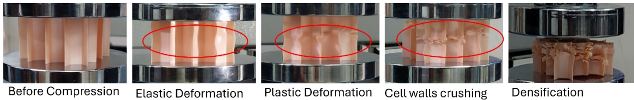
Figure 18: The failure mechanism of honeycomb structure from initiation to propagation
