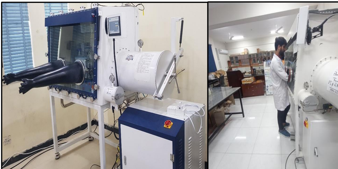
Figure 3.11: Coin cell fabrication process in a glove box.
