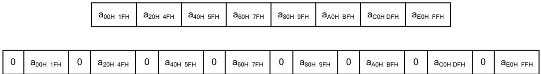
Figure 13.15 Interleaved zeros for warp scan.
