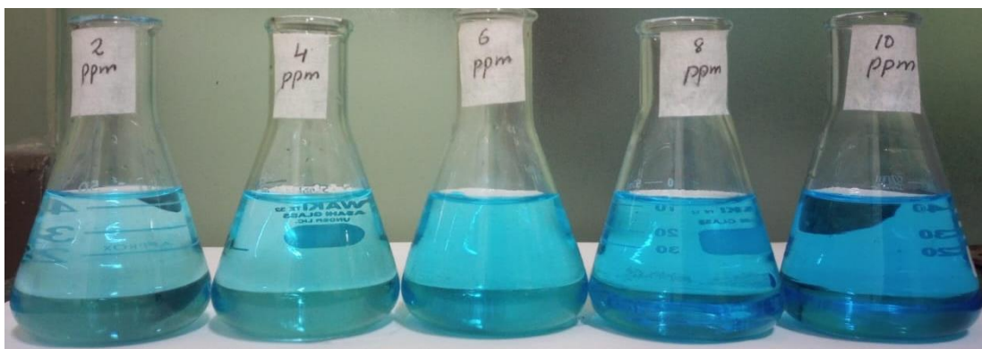
Figure 3.6: Preparation of methylene blue solutions for standard calibration curve
