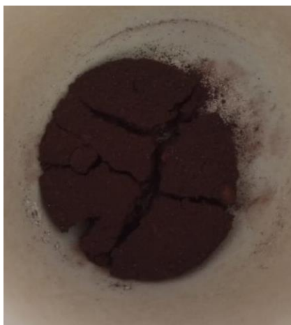
Figure 3.4: Synthesized zinc ferrite particles via coprecipitation route
