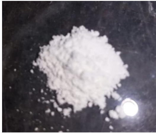
Figure 3.2: Synthesized zinc oxide particles via co-precipitation route
