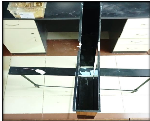
Figure 2.9. The Elevated Plus Maze: This test is conducted to assess anxiety-related behavior in mice. This test involves a plus-shaped apparatus with two open arms and two closed arms elevated above the ground. The time mice spend in the open arms versus the closed arms is measured. This assessment provides valuable insights into the effects of experimental treatments or conditions, such as stress or neurological disorders, on anxiety and exploratory behavior in mice.
