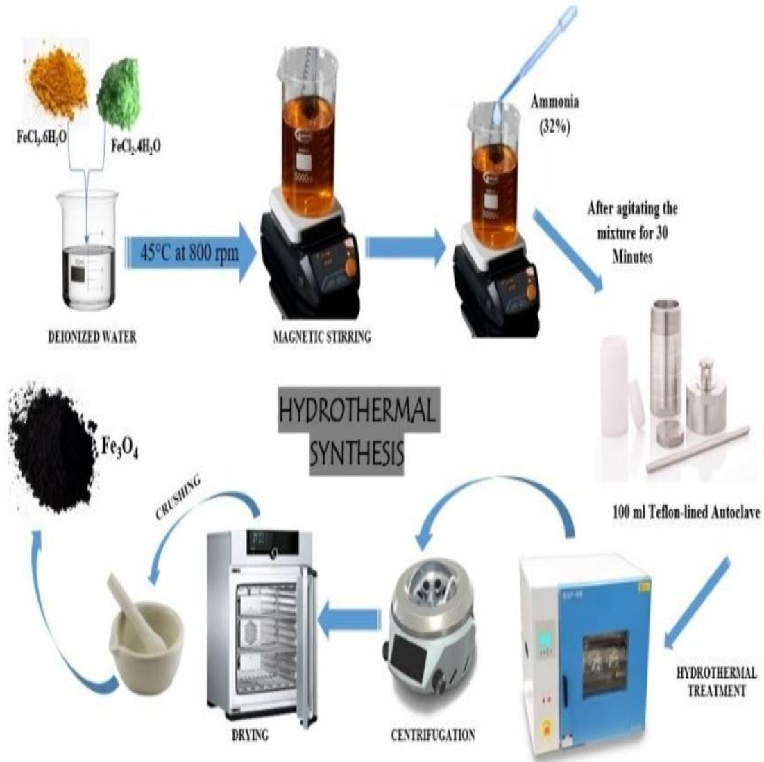
**Figure 3.6:** Hydrothermal synthesis process of  $\text{Fe}_3\text{O}_4$
