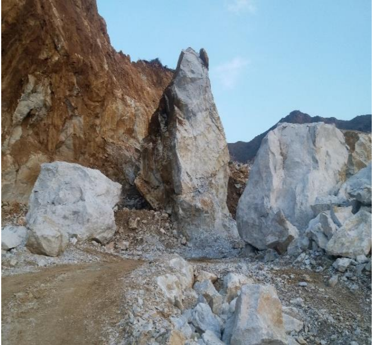
Figure 2-5: Non-Mechanized Marble Extraction
