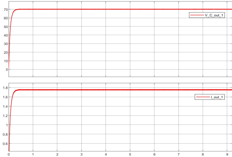
Figure 5.2(a): Voltage and current of first module of DC microgrid under buck mode.
