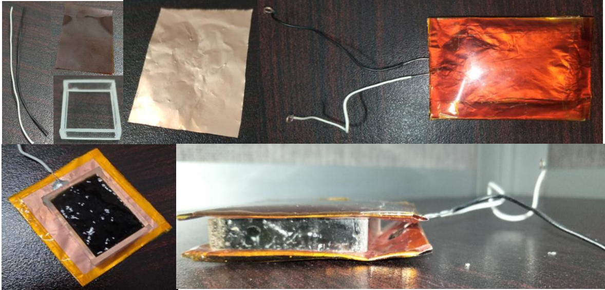
Figure 3.2: Device Fabrication (a) Device Parts including wires, acrylic framework, copper foil and Kapton Sheet (b) & (c) Assembled TEC (c) Gel Polymer Electrolyte in framework.
