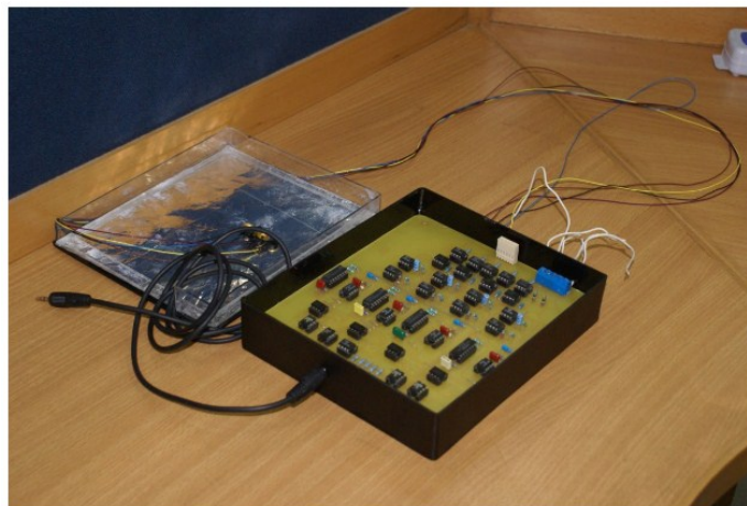
Figure 4.1 –EEG Signal Acquisition Device
