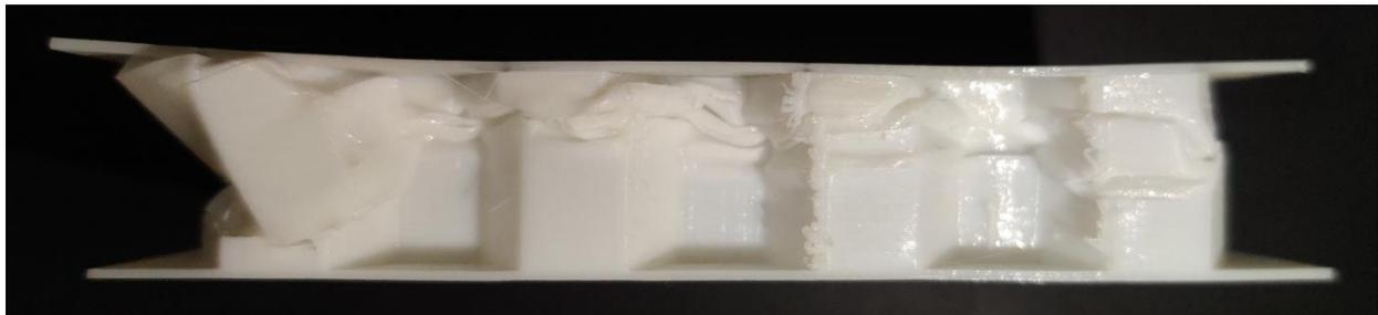
Figure 22: Deformation pattern of (TH) structure after compression
