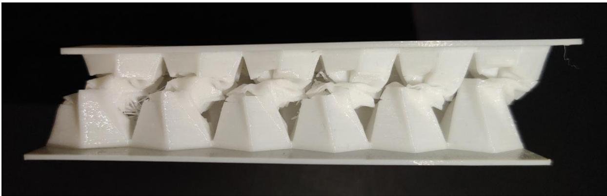
*Figure 23: Deformation pattern of (OH) structure after compression*
