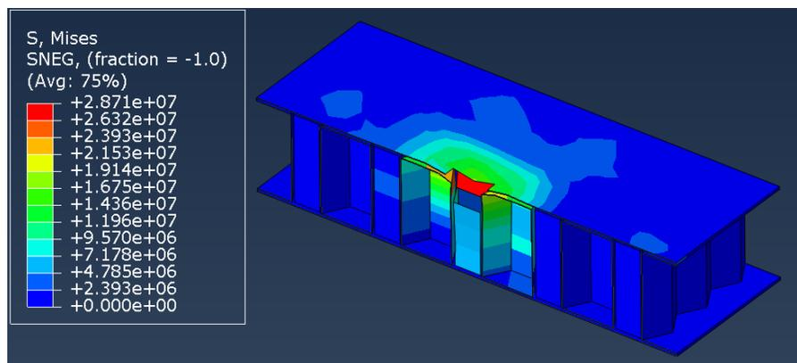
Figure 19: Von Mises stress distribution in (TH) structure during impact simulation
