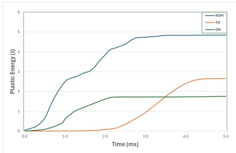
Figure 17: Comparison of Plastic energies of (TH), (OH), and (MOH) honeycomb structures under impact loading.
