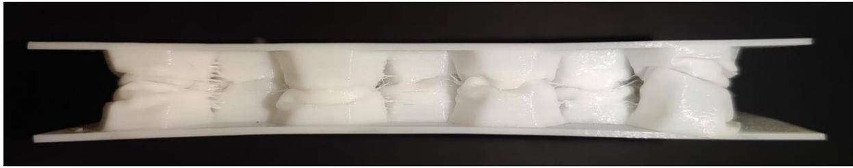
Figure 24: Deformation pattern of (MOH) structure after compression
