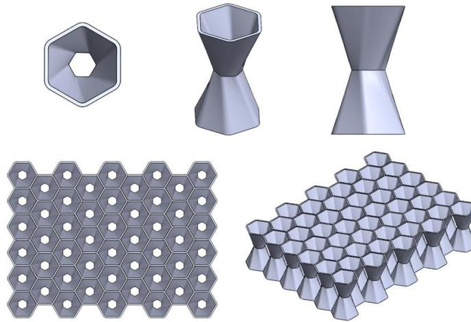
*Figure 8: Geometric specifications and dimensioning of Modified Origami Honeycomb (MOH) structure*
