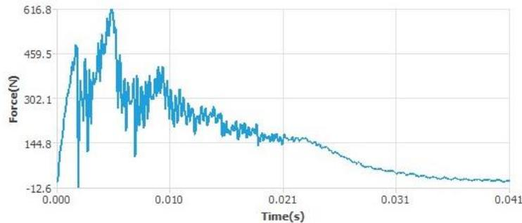
Figure 16: Force-time response of (MOH) structure under drop weight
