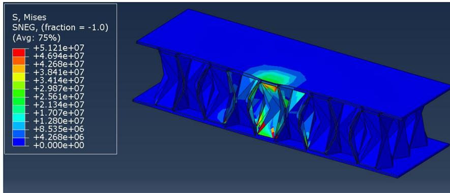
Figure 20: Von Mises stress distribution in (OH) structure during impact simulation
