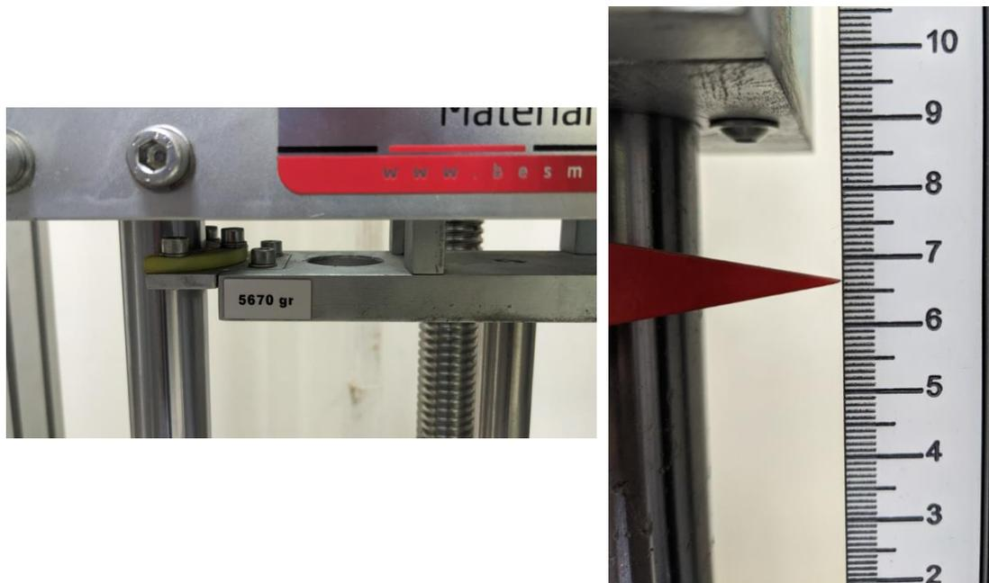
*Figure 13: Drop weight test configuration*
