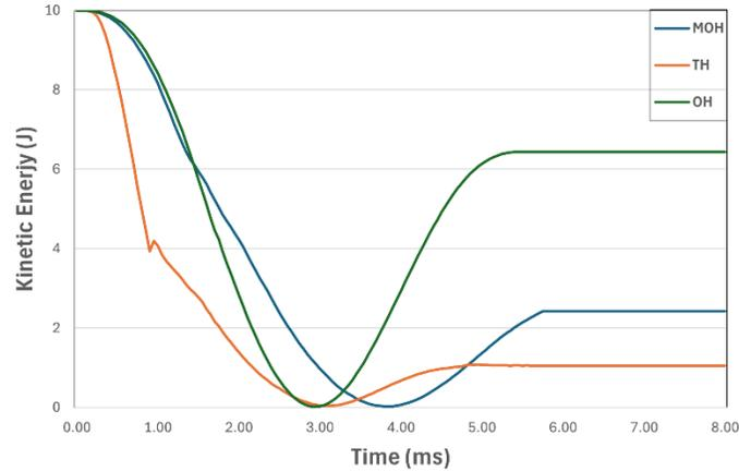
Figure 18: Comparison of kinetic energies of (TH), (OH), and (MOH) honeycomb structures under impact loading.
