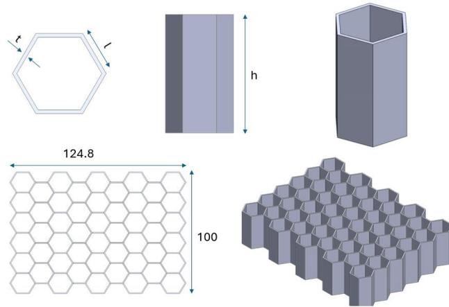
Figure 6: Geometric specifications and dimensioning of Traditional Honeycomb (TH) structure
