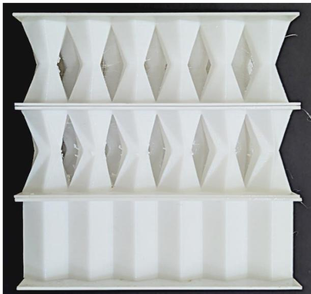
*Figure 9: 3D-printed prototypes of (TH), (OH), and (MOH) structures fabricated.*
