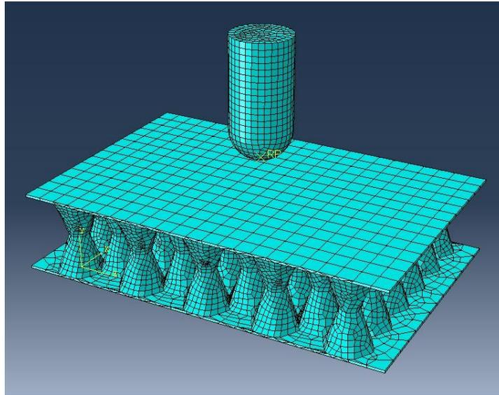
Figure 11: Mesh generation of honeycomb structure and impactor using S4R shell elements in Abaqus.
