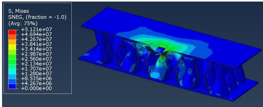
Figure 21: Von Mises stress distribution in (MOH) structure during impact simulation
