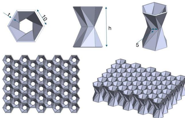
Figure 7: Geometric specifications and dimensioning of Origami Honeycomb (OH) structure
