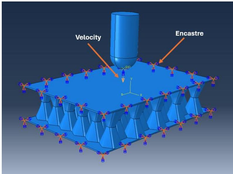
*Figure 10: Boundary conditions applied to honeycomb structure in Abaqus/Explicit finite element model.*
