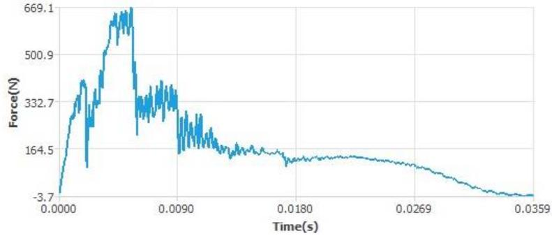
Figure 15: Force-time response of (OH) structure under drop weight
