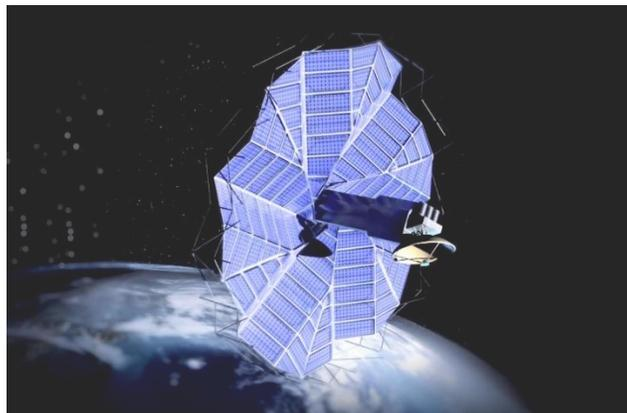
*Figure 1: Miura-Ori fold application in space industry.*
