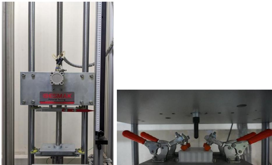
*Figure 12: BESMAK drop weight impact testing machine configured according to ASTM D7136 standard.*
