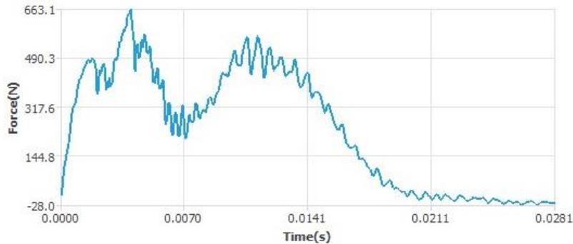
Figure 14: Force-time response of (TH) structure under drop weight
