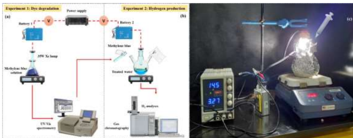
Figure 3.2: Experimental setup of photocatalytic dye degradation and hydrogen production
