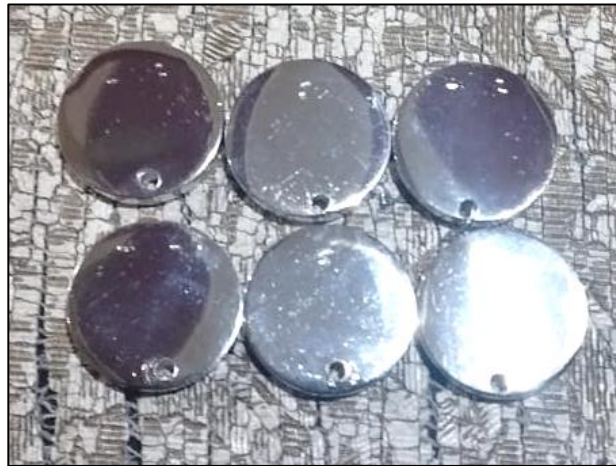
Figure-7: Nickel electroplated Specimens (Sample type-4)
