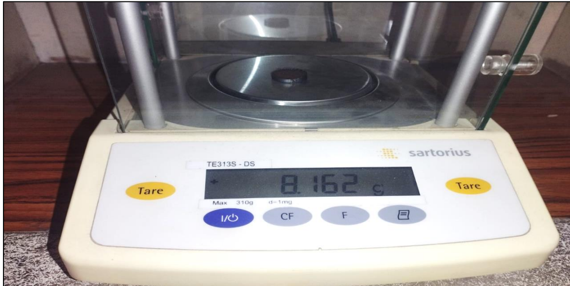
Figure -12: Sartorius Model TE313S-DS Electronic Analytical and Precision Metal Scale
