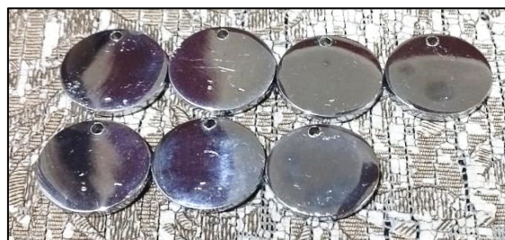
Figure -8: Dual coated (Ni-Cr) Specimens (Sample type-5)
