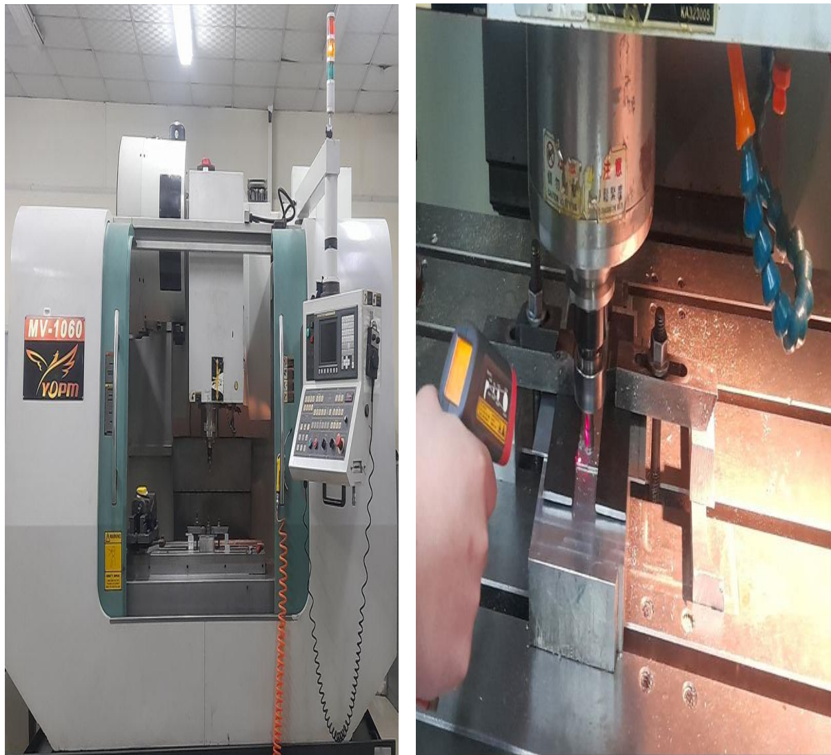
Figure 17: (a) Vertical CNC Milling (b) FSW Set up
