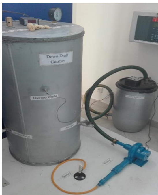
Figure 3-5: Downdraft Biomass Gasifier Unit
