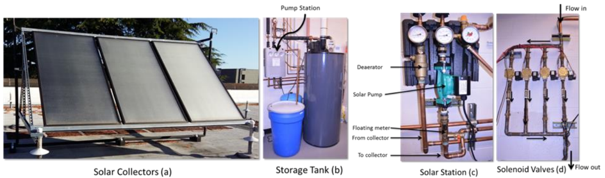
Figure 1-4 : Components of the SWHs in TEST lab
