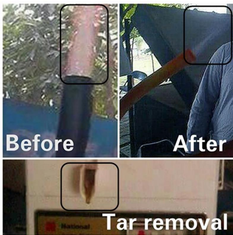
Figure 4-4: Difference b/w flame qualities before and after tar removal.
