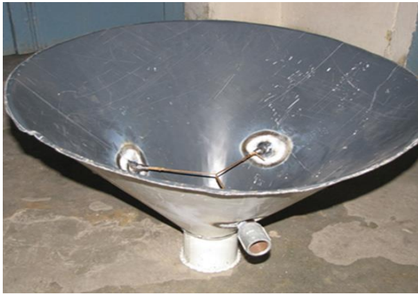
Figure 3-3: Throat of Gasifier and Nozzles Fixing
