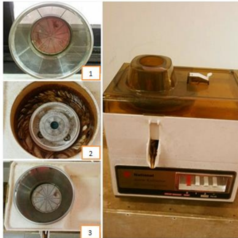
Figure 3-9: Parts of scrubber and picture of inside story for tar removal
