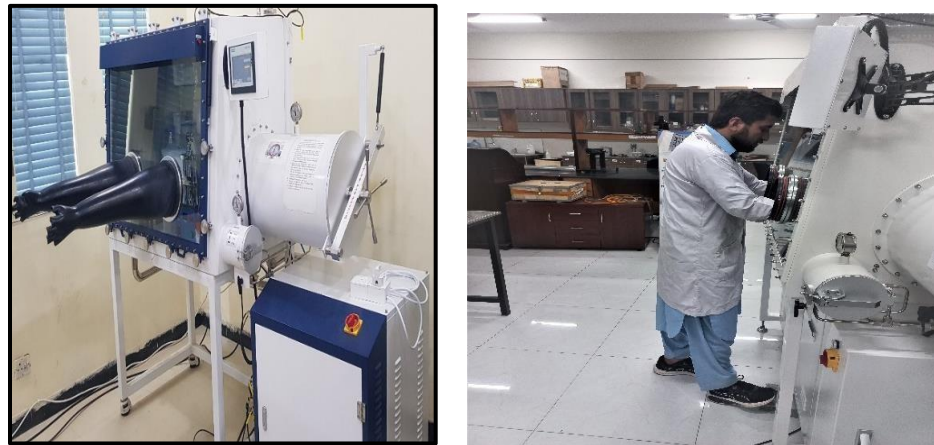
Figure 3.8: Images shows cutting electrodes and the fabrication and assembly of coin cell in the glove box.
