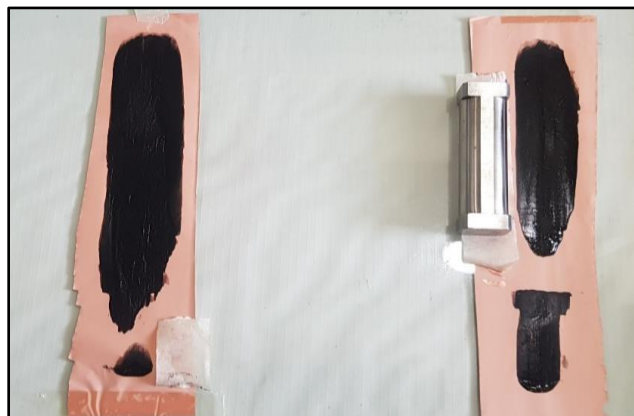
Figure 3.6: Images shows the the pasting of slury on copper foil by using doctor blade.
