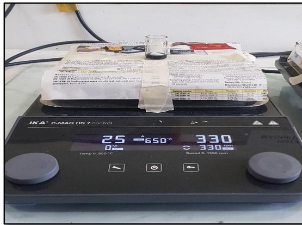
Figure 3.5: Image shows the mixing of active material with binder carbon black on the magnetic stirring.
