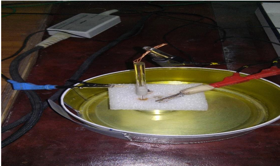
Figure 4.7: Schematic Diagram of Three Electrodes Setup
