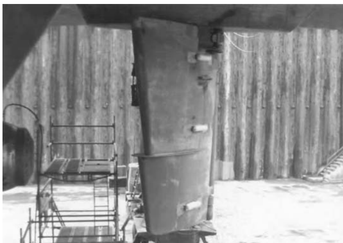
Fig. 21.1 Profile of a twisted rudder.
