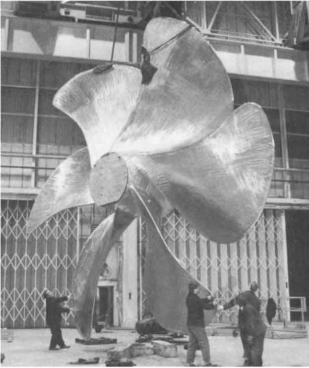
Fig. 9.3 A large modern container ship propeller nearing completion. This 70 tonnes screw has a diameter of 8550 mm and is designed to absorb 42.5 MW at 94 r/min.
