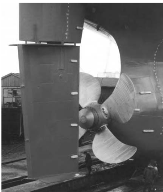
Fig. 21.2 A Schilling rudder.
