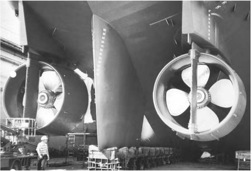
Fig. 21.13 Vessel with Twin Kort steering nozzles and Becker flaps.
