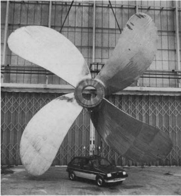
Fig. 9.4 The economy propeller, with a finished weight of 69 tonnes and a diameter of 11 m, before retrofit to a 320 ktonnes dwt ULCC. Reference source: 'Developments in Marine Propellers' by Dr G. Patience for Institute of Mechanical Engineers (London) January 1991.
