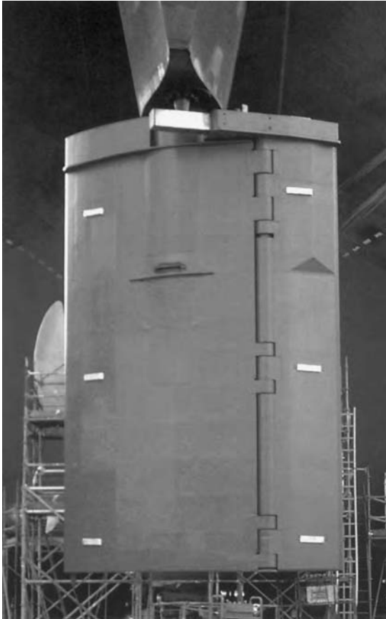
Fig. 21.11 Becker tail-flap rudder.
