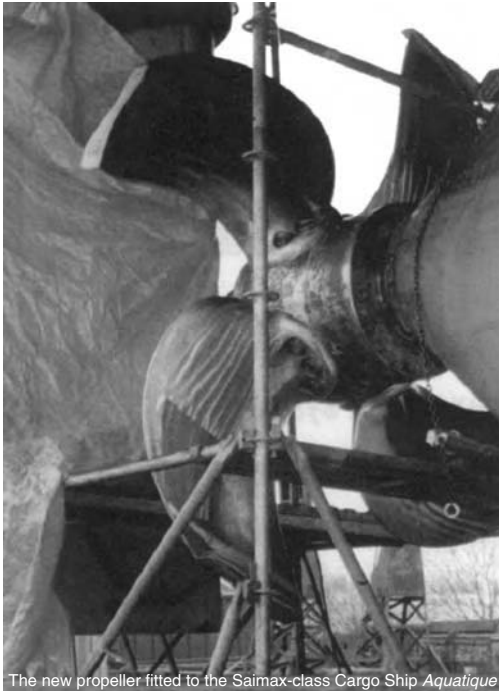
Fig. 22.5 The GPT tip-plate propeller design.
