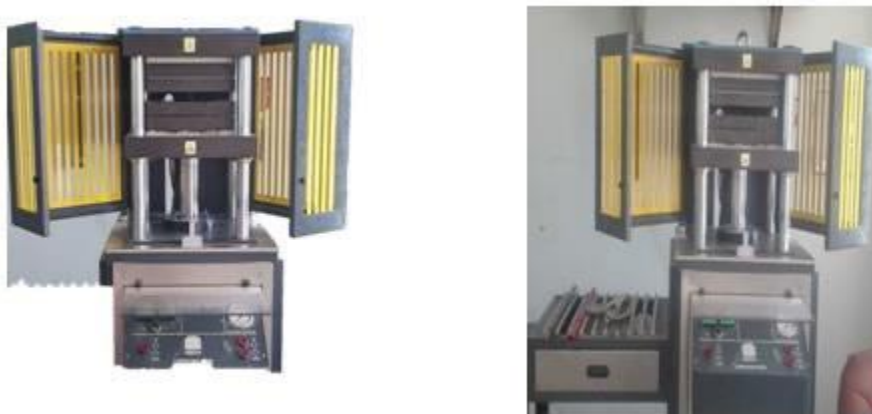
Figure 16: Hot presser used for making films
