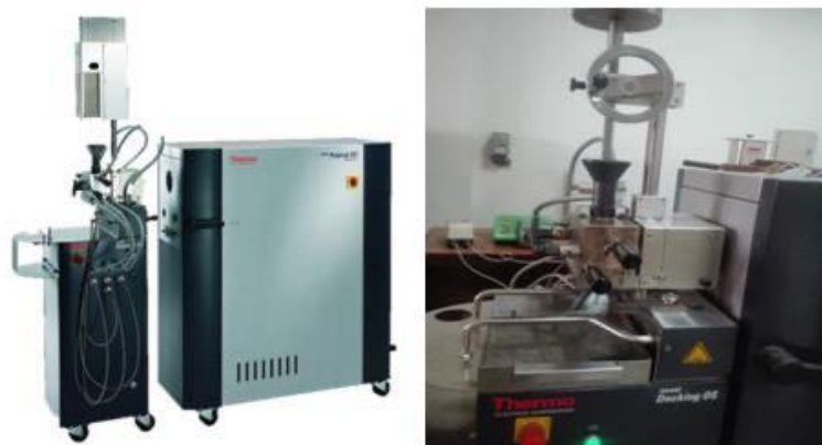
Figure 15: (a) Intense Mixer used for blending (b) HAAKE Intense Mixer at UET Lahore
