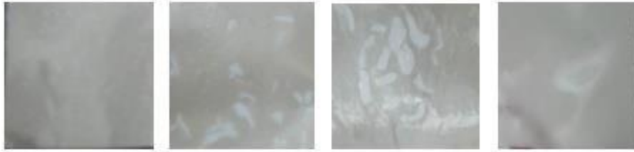
Figure 18: Films obtained after cold pressing a) F1: 80% PCL & 20 % CS b) F2 : 70% PCL & 30% CS C) F3: 60% PLA & 40% CS d) F4: 50% PCL & 50% CS
