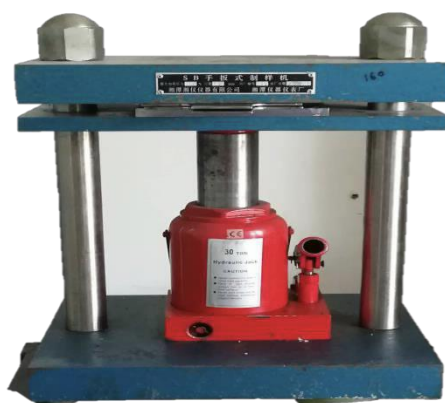
Figure 17: Cold presser used for making sheets
