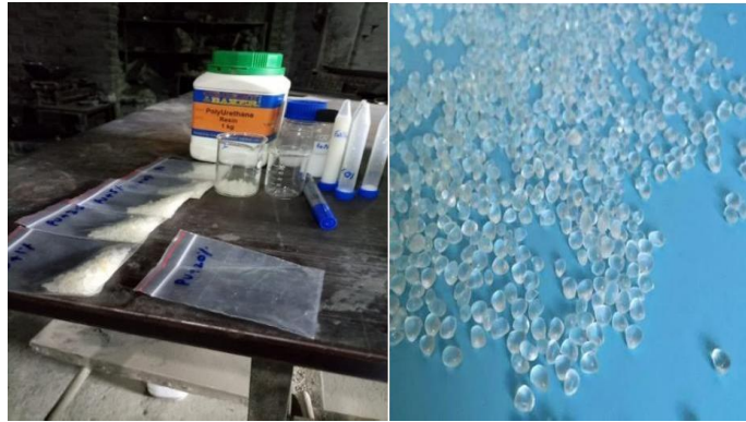
Figure 3. 4: Samples with different composition of emulsion(a) and Polyurethane resin (pallet)(b)
