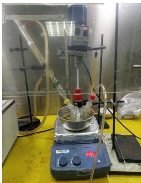
Figure 3. 1: Set-up for emulsion polymerization composed of nitrogen inlet, condenser, thermometer and magnetic stirrer.
