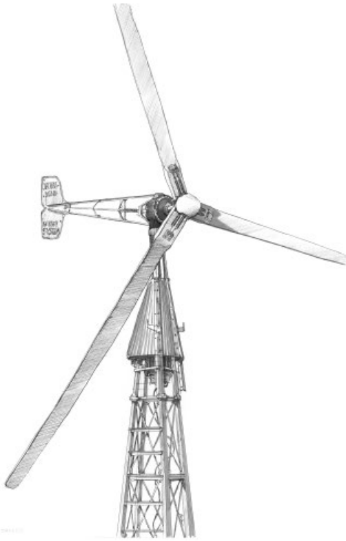
Figure 2.1 A 2.5-kW Jacobs wind turbine. The small wind turbines built by Marcellus and Joe Jacobs represented the state of the art in the 1930s and 1940s. The Jacobs wind turbines contained more features and were more expensive than others, which earned them the reputation as the “Cadillac” of small wind turbines.
