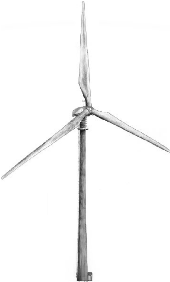
Figure 17.1 Kenetech's KVS-33 wind turbine was a 300-kW variable-speed machine. After sinking millions in its development, Kenetech's fortunes sank when initial versions of the wind turbine proved to be unreliable.
