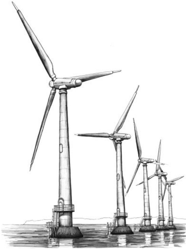
Figure 20.1 Built in 1991, the Vindeby Offshore Wind Farm in Denmark was the world's first. The wind farm used 11 Bonus B35/450 kW wind turbines for a total installed capacity of 4.95 MW. The turbines were modified for offshore use by sealing the towers.
