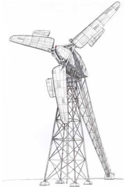
Figure 3.1 The Soviet Union's 100-kW wind turbine at Balaklava in the Crimea. It was the first 100-kW wind turbine ever built and it was successfully interconnected to the local transmission network and co-dispatched with an existing thermal power plant. It was likely destroyed in 1942 when the Russians defended Sevastopol from the Germans.
