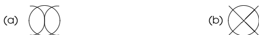
Figure 1.5 (a) Midships symbol in English literature, (b) Midships symbol in German literature
