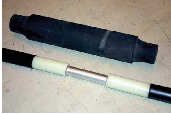
Fig. 4.4 Pre-moulded polymeric cable joint. The elastomeric joint sleeve on top . Conductor connected and insulation prepared for application of insulation sleeve on bottom
