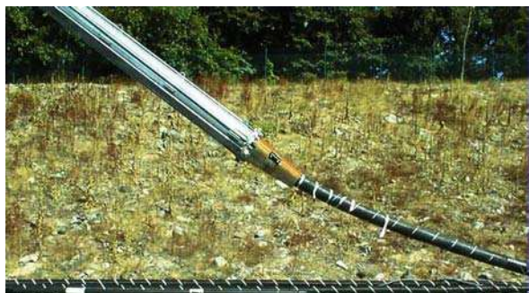
Fig. 4.3 Rigid submarine installation joint in a steel casing for a 1C cable during an on-shore bending test
