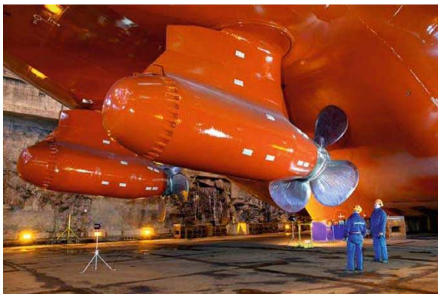
Fig. 7.8 Azimuth pods (Courtesy of ABB Oy, Marine, Finland)
