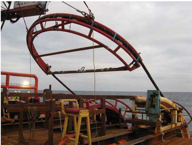
Fig. 7.18 The quadrant, a steel support frame, goes into the water (Courtesy of ABB, Sweden)
