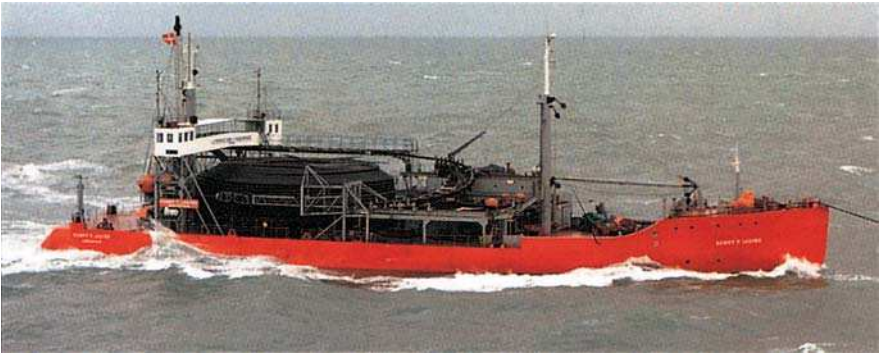
Fig. 7.4 Cable laying barge “H.P. Lading”. Tow barge with turntable for up-and-down spooling on the conical hub (Courtesy of NKT Cables A/S)
