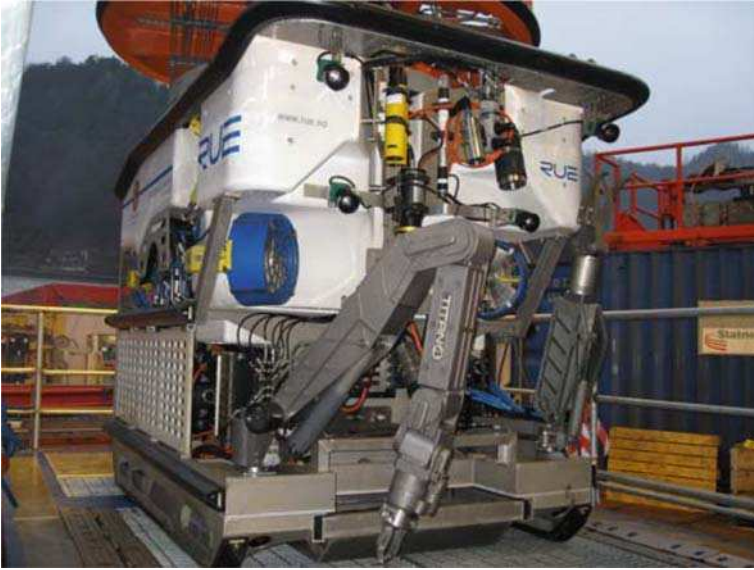
Fig. 7.11 ROV with grip manipulators and cameras
