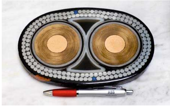
Fig. 2.10 Two core 450 kV HVDC cable for the NorNed project
