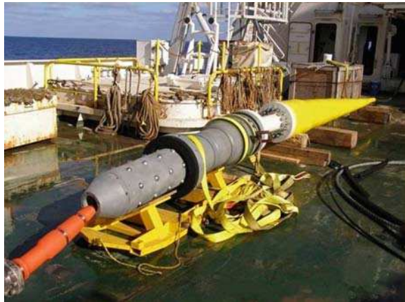
Fig. 4.10 Bending stiffener (right hand) together with a diverless subsea cable connector (left side). (Courtesy of Trelleborg, UK)
