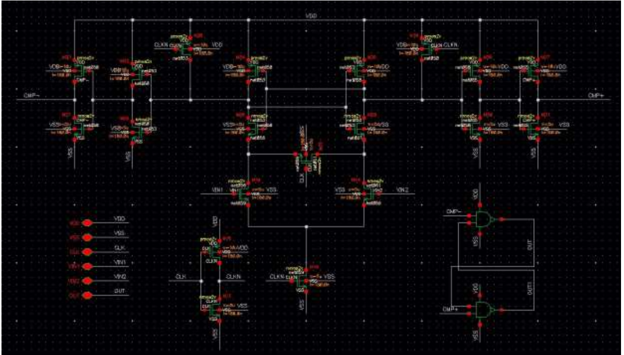
Figure 3.3: Dynamic Latch Comparator Schematic.
