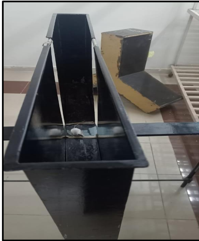
Figure 2.8: Elevate plus maze test. Anxiety-like behaviour in mice was evaluated using an EPM apparatus, which measured the amount of time spent in open versus closed arms.
