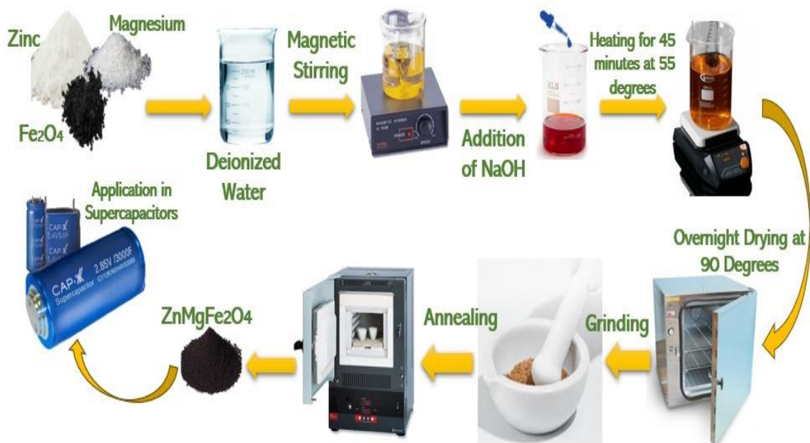
Figure 0.1: Synthesis of Ferrites Via Coprecipitation.
