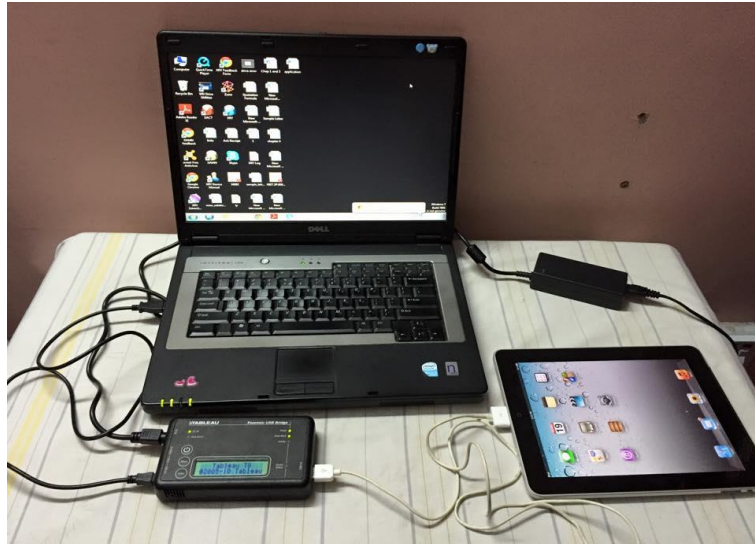
Figure 6.3: Device Detect LED of Forensic USB Bridge does not Give Steady Illumination when Connected to iPad.
