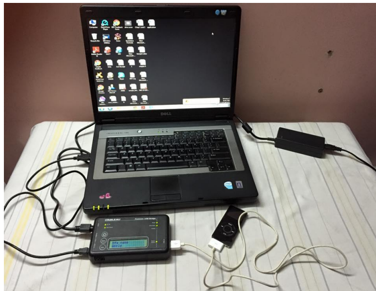
Figure 6.4: Device Detect LED of Forensic USB Bridge Gives Steady Illumination when Connected to iPod.
