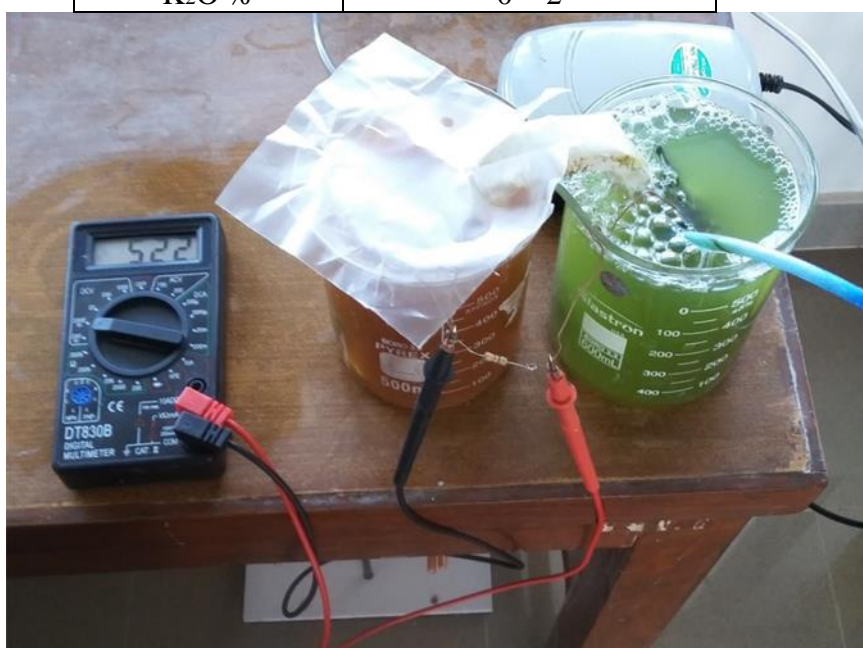
Figure 19 The yeast based MFC showing 522 mV of Open Circuit Voltage
