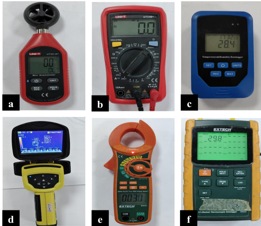
Figure 3. 11: (a) An anemometer measures wind velocity produced by the intake fan at the top side. (b) A digital multimeter measures the current voltage of the AWH system. (c) Temperature and Humidity sensors Measure the temperature and relative humidity (d) IR camera provides temperature profile (e) Clamp meter measures the electrical consumption (f) temperature datalogger for measuring temperature
