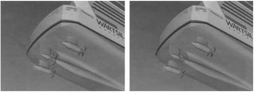
Fig. 22.10 An impression of the CODED hybrid propulsion system in action: in high-speed mode (left) and low-speed mode (right) with the centre propeller feathered.
