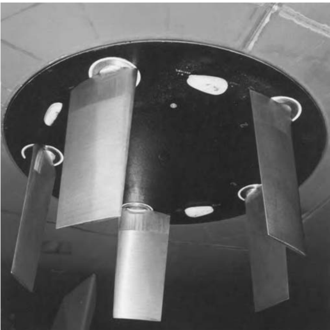
Fig. 22.1 VSP units. Blade depth indicated by height of man. Bottom of shell plating is shown in (b).
