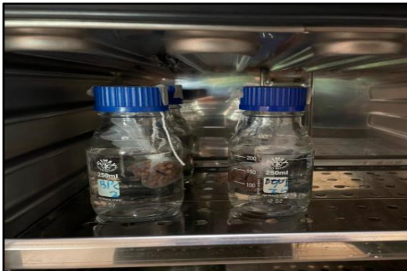
Figure 5: Water release test of urea, BPU and DCRFs at 25°C according to (ISO (18644-2016)). A nylon bag containing the fertilizer, suspended in 200ml of DI water to assess the release patterns of nitrogen and zinc
