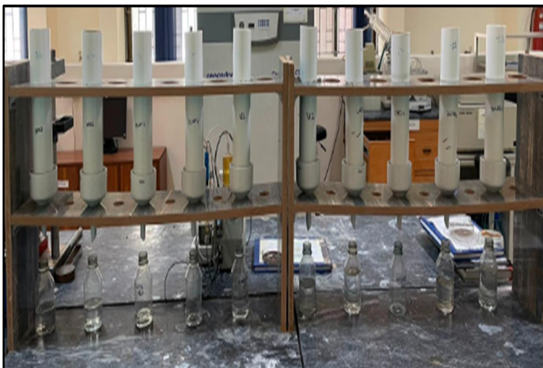
FIGURE 6: Sand column testing of urea, BPU and DCRFs as reported by (Fachini et al., 2022) – fertilizers were kept between the layers of washed sand and 200ml DI water is passes through it on daily basis and the leachate is assessed for nitrogen and zinc release concentrations.
