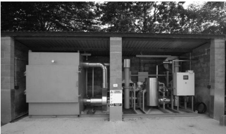
Figure 2.3 A batch fed pilot scale slow pyrolysis unit, located at the Institute for Biological Environmental and Rural Sciences at Aberystwyth University ( http://beaconwales.org/ ).
