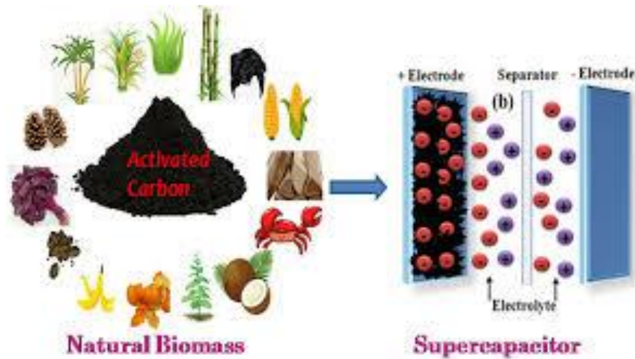
Figure 10: Biomass derived activated carbon as supercapacitor electrode [42].
