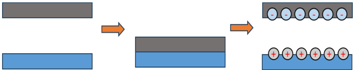
Figure 1.7: Schematic of Material Transfer in TENG.
