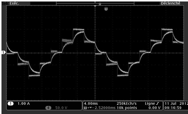
Figure 5.11. Output voltage and current (after appropriate resizing) in the circuit (for a color version of this figure, see www.iste.co.uk/fribourg/switchingsystems.zip )
