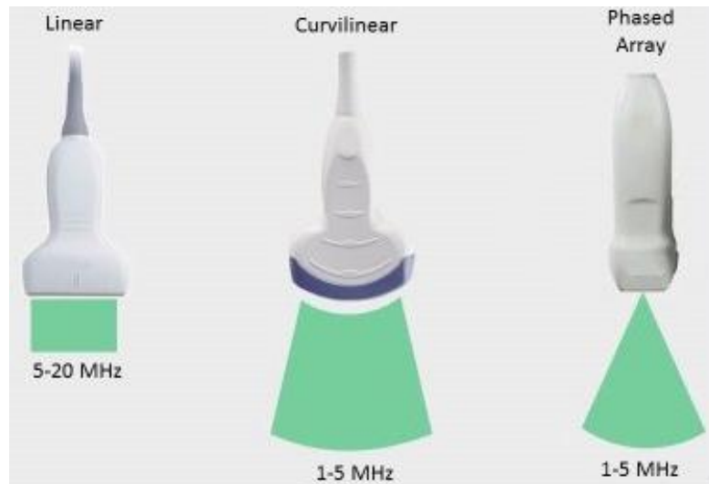
Figure 6: Linear vs Curved vs Phased Array Transducers
