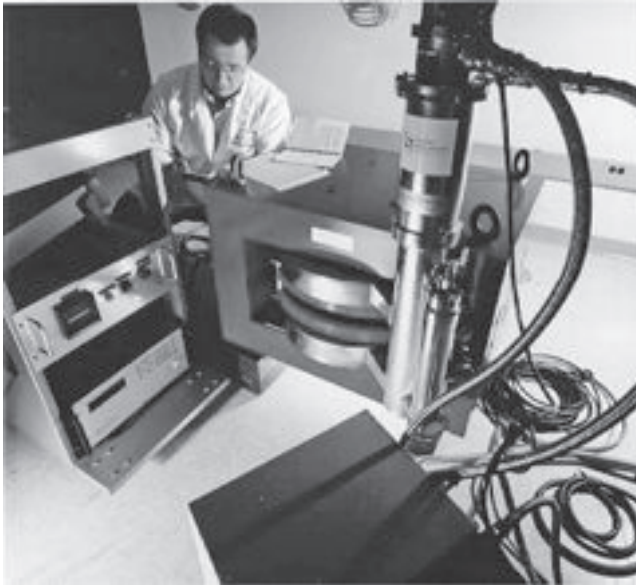
Figure 11.6 Magnet assembly showing major components such as iron core, HTS coil cryostat, cryocooler, and power supply (Courtesy of American Superconductor Corporation)
