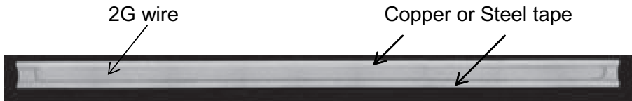
Figure 2.11 American Superconductor Corporation 344 conductor—2G conductor sandwiched between copper tapes
