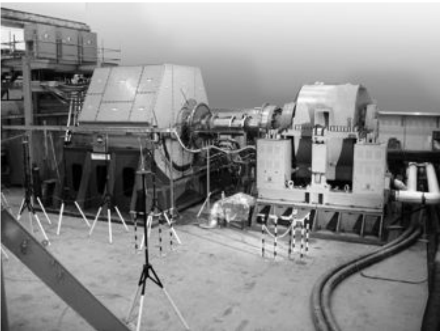
Figure 4.21 AMSC's 36.5-MW motor undergoing factory testing (Courtesy of American Superconductor Corporation)
