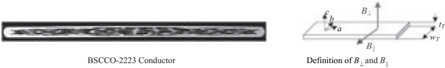
Figure 2.5 Cross section of a typical BSCCO-2223 conductor of 0.2\text{ mm} \times 4\text{ mm} (Courtesy American Superconductor Corporation)
