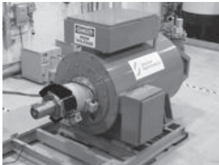
Figure 4.19 AMSC's 5000-hp, 1800-RPM synchronous motors employing HTS field windings tested in 2001 (Courtesy of American Superconductor Corporation)
